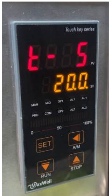
In order to hold 1240c for 20 minutes we set t -5 as 20
