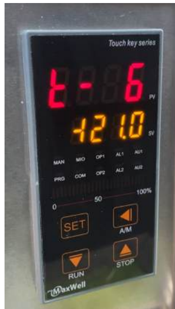
Finally we want the kiln to 'STOP' So for t-6 we enter -121.0 which is the stop instruction for the kiln.
