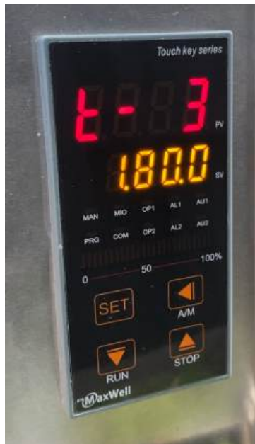
t - 3 has been set as 180 minutes so the kiln will take 180 minutes to get from 1000c 1180c
