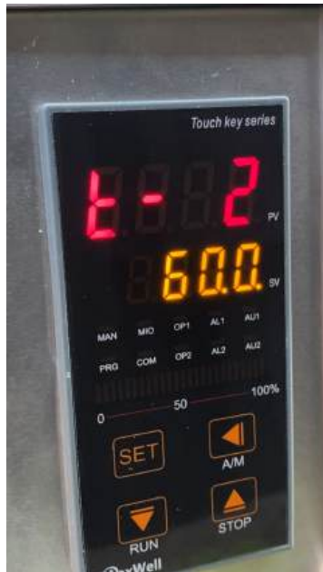
T - 2 has been set as 60 minutes so the kiln will spend 60 minutes getting to 1000c
