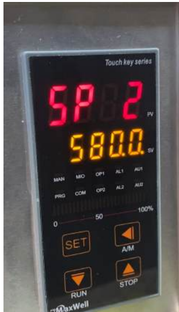
Above second set point (sp2 has been set to 580 degrees celsius.
